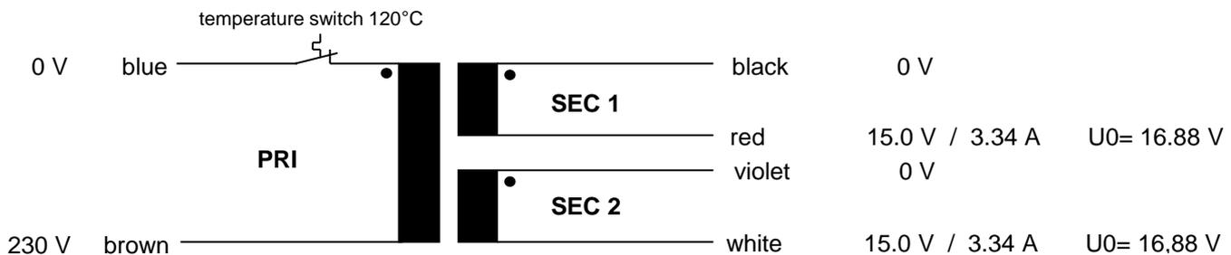
possible connection: parallel connection **15.0V / 6.68A** = connect black with violet and red with white
